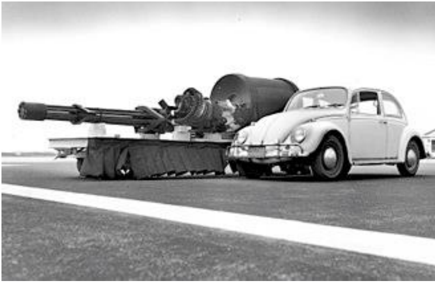
A 7-barrelled Gatling Gun with its firing mechanism and ammunition drum, removed from its A-10 aircraft, compared for size with a VW Beetle car. (US Airforce photo)
